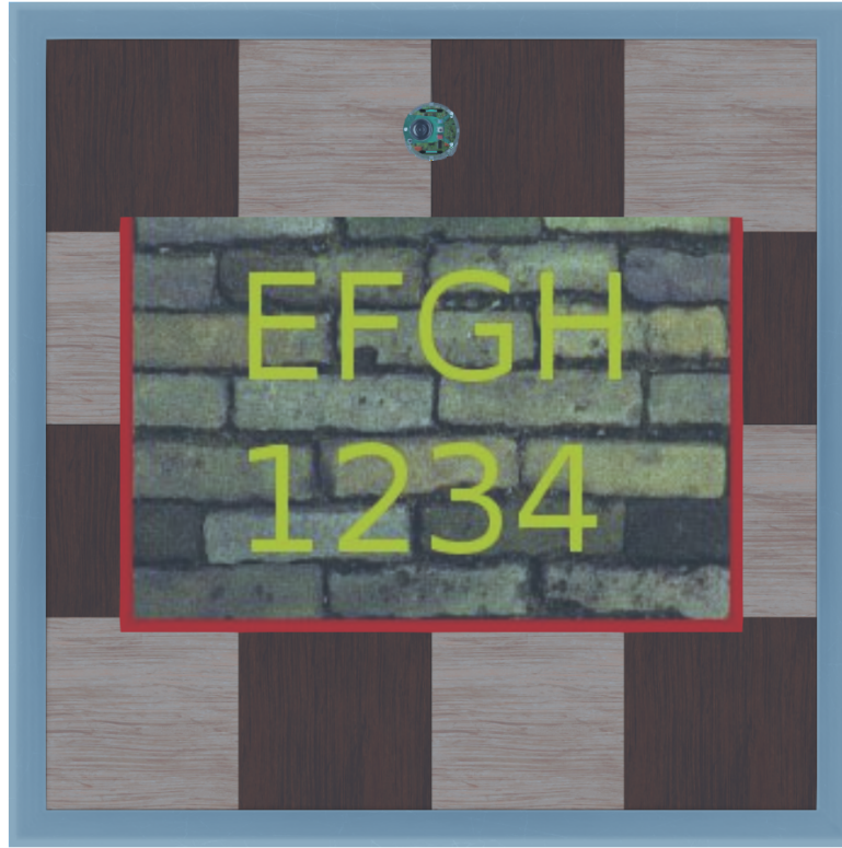
Figure 25: Top view of the arena used for the collision avoidance task. The big object with the writings in the center is the obstacle that the robot have to circumnavigate.
